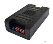
The PS-BG216 is a fully regulated switch mode power supply providing 12 Volts DC at 8 Amps. The high frequency action enables it to work smoothly on a very wide AC input voltage range from 120 to 280 Volts with comparatively low power losses, high efficiency small size and lesser weight. Application: For 16 IR Camera up to 24 Led.
