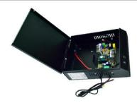
The PS0212CPSMSC is a fully regulated switch mode power supply providing 12 Volts DC at 2 Amps along with the facility of charging the battery for back up. The high frequency action enables it to work smoothly on a very wide AC input Voltage range from 120 to 280 Volts with comparatively low power losses, high efficiency, small size and lesser weight.
