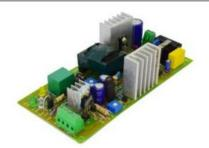
The PS0412C is a fully regulated switch mode power supply providing 12 Volts DC at 4 Amps along with the facility of charging the battery for back up. The high frequency action enables it to work smoothly on a very wide AC input Voltage range from 120 to 280 Volts with comparatively low power losses, high efficiency, small size and lesser weight.
