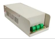
The PS0412N-IAS is a fully regulated switch mode power supply providing 12 Volts DC at 4 Amps. The high frequency action enables it to work smoothly on a very wide AC input Voltage range from 120 to 280 volts with comparatively low power losses, high efficiency small size and lesser weight.
