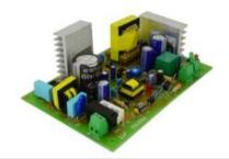
The PS0512C is a fully regulated switch mode power supply providing 12 Volts DC at 5 Amps along with the facility of charging the battery for back up. The high frequency action enables it to work smoothly on a very wide AC input Voltage range from 120 to 280 Volts with comparatively low power losses, high efficiency, small size and lesser weight.
