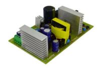
The PS0524C is a fully regulated switch mode power supply providing 24 Volts DC at 5 Amps along with the facility of charging the battery for back up. The high frequency action enables it to work smoothly on a very wide AC input Voltage range from 120 to 280 Volts with comparatively low power losses, high efficiency, small size and lesser weight.
