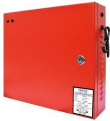
The PS0524CPSMSC is a fully regulated switch mode power supply providing 24 Volts DC at 5 Amps along with the facility of charging the battery for back up. The high frequency action enables it to work smoothly on a very wide AC input Voltage range from 120 to 280 Volts with comparatively low power losses, high efficiency power supply.
