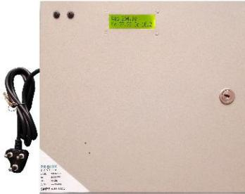
The PS0624N-LCD is a fully regulated switch mode power supply with live display output current, volt and input AC providing 24 Volts DC at 6 Amps. The high frequency action enables it to work smoothly on a very wide AC input Voltage range from 120 to 280 volts with comparatively low power losse
