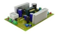
The PS10A12C is a fully regulated switch mode power supply providing 12 Volts DC at 10 Amps along with the facility of charging the battery for back up. The high frequency action enables it to work smoothly on a very wide AC input Voltage range from 120 to 280 Volts with comparatively low power losses, high efficiency, small size and lesser weight.
