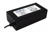
The PS12-12CNTR is a fully regulated switch mode power supply providing 12 Volts DC at 3 Amps. The high frequency action enables it to work smoothly on a very wide DC input Voltage range from 10 to 14 volts with comparatively low power losses, high efficiency small size and lesser weight
