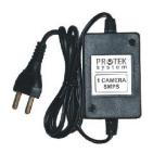
The PS1CPS is a fully regulated switch mode power supply providing 12 Volts DC at 750mAh. The high frequency action enables it to work smoothly on a very wide AC input voltage range from 90 to 280 Volts with comparatively low power losses, high efficiency small size and lesser weight. Application: For 1 IR Camera up to 24 Led.
