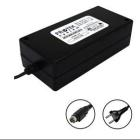
The PS312-HIK is a fully regulated switch mode power supply providing 12 Volts DC at 3 Amps. The high frequency action enables it to work smoothly on a very wide AC input Voltage range from 90 to 280 volts with comparatively low power losses, high efficiency small size and lesser weight. Application For 8CH & 16CH Hikvision DVR
