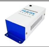
The PS4CPS is a fully regulated switch mode power supply providing 12 Volts DC at 2 Amps. The high frequency action enables it to work smoothly on a very wide AC input voltage range from 90 to 280 Volts with comparatively low power losses, high efficiency small size and lesser weight. Application: For 4 IR Camera up to 24 Led.
