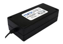
The PS512NABS is a fully regulated switch mode power supply providing 12 Volts DC at 5 Amps. The high frequency action enables it to work smoothly on a very wide AC input Voltage range from 90 to 280 volts with comparatively low power losses, high efficiency small size and lesser weight. Application For 8-10 Nos CMount/Dome Cameras/16CH DVR
